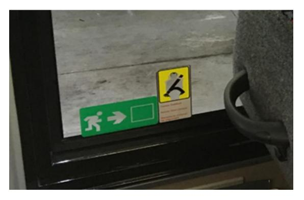
Some secondary manufacturers of limousines and custom coaches are placing red lights over emergency exit windows in lieu of the designation marking. This may be done in addition to the required labeling but does not meet the marking requirements in FMCSRs/FMVSS.
