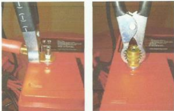
Correct Charge or Test Cable Clamp Connections
